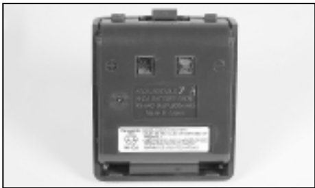
PART NO.: BATT-A40 3.6V 600MAH NI-CAD PANASONIC KX-A40 KX-T9020
